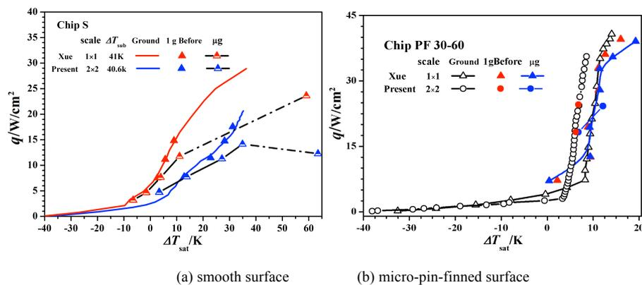
Fig. 1 Heater size effect on boiling heat transfer in normal gravity and microgravity
